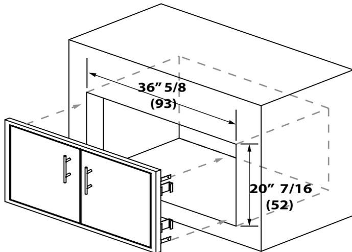
ATORNILLAR Ó PIJAR LAS ANCLAS EN LAS PAREDES LATERALES DEL HUECO
